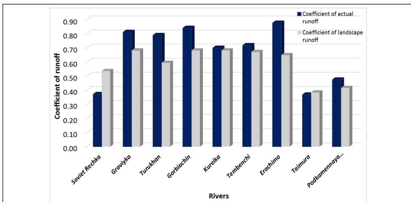
**Figure 3:** Comparison of the runoff coefficient (actual and calculated) for the different catchments under study. Runoff coefficient is the ratio of the total runoff to the sum of precipitation for the same period.
