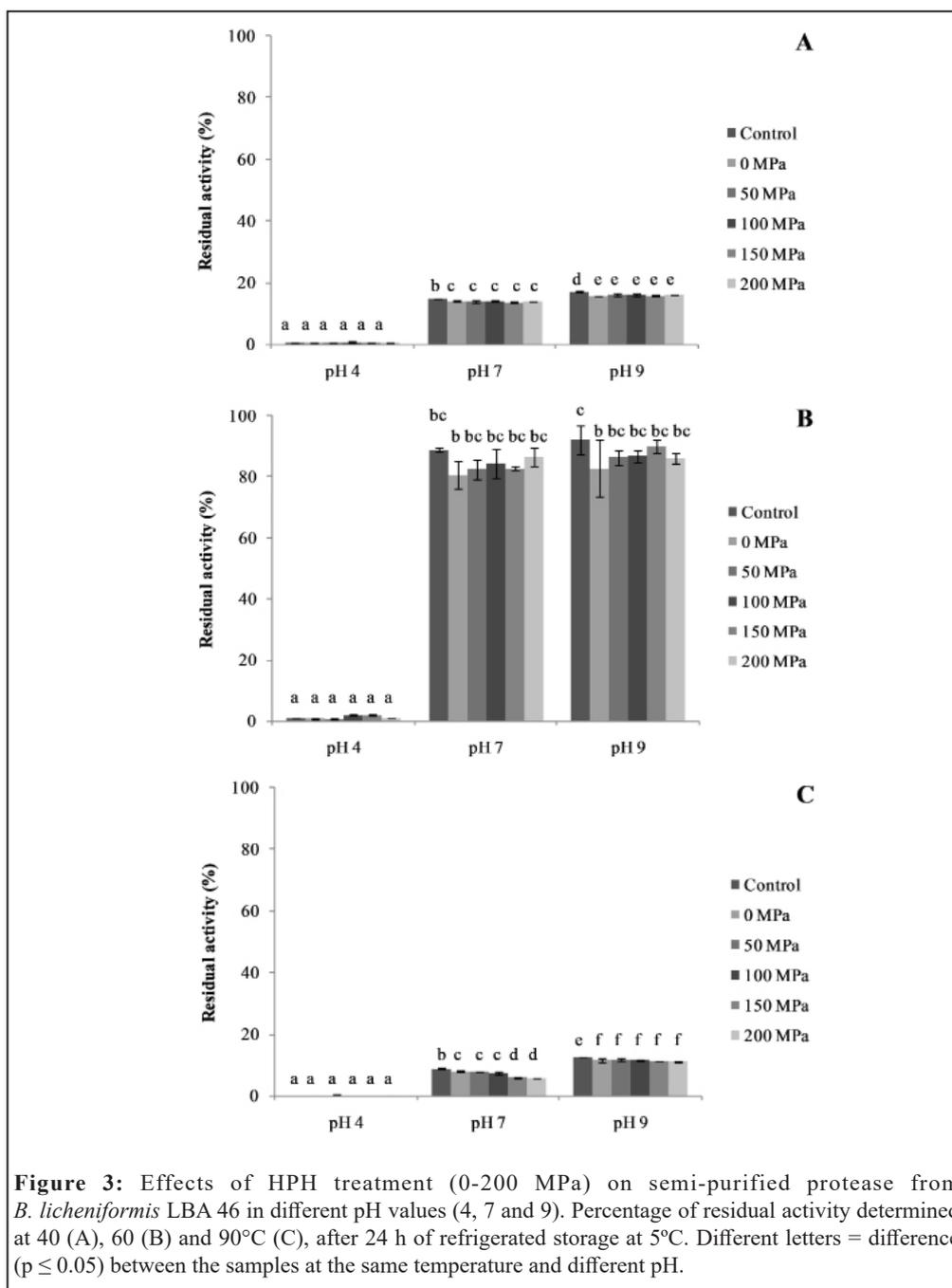
**Figure 3:** Effects of HPH treatment (0-200 MPa) on semi-purified protease from *B. licheniformis* LBA 46 in different pH values (4, 7 and 9). Percentage of residual activity determined at 40 (A), 60 (B) and 90°C (C), after 24 h of refrigerated storage at 5°C. Different letters = difference ( $p \leq 0.05$ ) between the samples at the same temperature and different pH.
